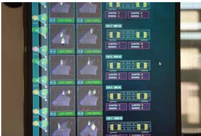
Figure 4: Dwell Track™ technology showing real time tracking of passengers
