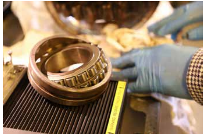
Figure 2: Researchers at the University of Queensland assessing lubrication regimes on in-service axle bearings.
